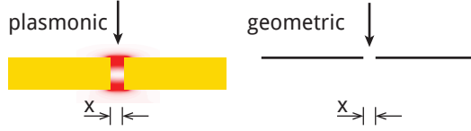
Figure 2.20: Geometry for plasmonic metal-insulator-metal (left) and geometric toy model (right) transduction.
