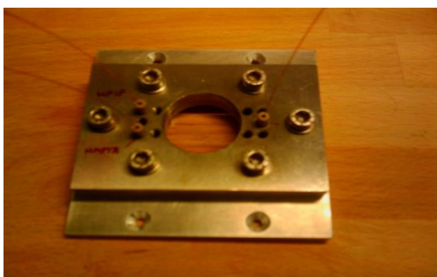
Figure s2. The lab-on-a-chip in a chip holder
