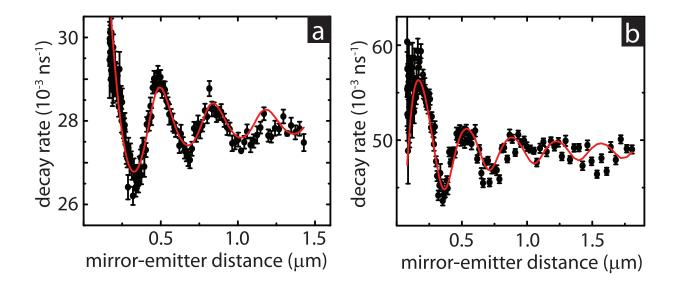
FIG. 3. (a) Data-points: Decay rate of a single NV center in a diamond nanocrystal as a function of distance to the scanning mirror. Error bars denote  $1\sigma$ -interval. Red solid line: Calculation of LDOS experienced by emitter at depth d = 150 nm into the substrate, with dipole moment in the sample plane ( $\theta = 0^{\circ}$ ) and QE = 26%. (b) Same as (a) but for NV defect in different nanocrystal (Calculation: QE = 58%).
