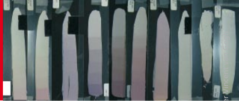
Fig. 5. Influence of thickness in transparent lake paints on fading; a, b) B2LW, before and after ageing; c, d) EOLW, before and after ageing. Composition of photographs K.J. van den Berg.
