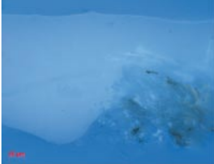
Fig. 2. Cross-section of the ground reconstruction at 200x magnification, bottom layer only (no top layer was added over this part). The thin layer fluorescing at the surface is oil which has separated out of the chalk/oil mixture. This indicates that the fluorescing layer in the centre of Figure 1 is an oil layer due to binder separation.
