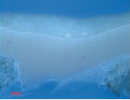
Fig. 1. Cross-section of ground reconstruction in ultraviolet light (200x magnification). Bottom layer is chalk (calcite) with an oil binder (1:1 mixture of raw linseed oil and litharge treated drying oil), top layer is stack method lead white with 7% by weight barium sulphate (no processing agents added). The layer in the centre is fluorescing and appears to be an oil layer. On an unknown sample, this could be interpreted as a deliberate addition of a thin layer of oil between ground layers.
