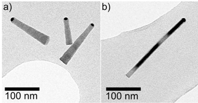
Figure 2. Transmission electron microscopy images of a) conical nanorods (sample I) and b) cylindrical nanorods.
