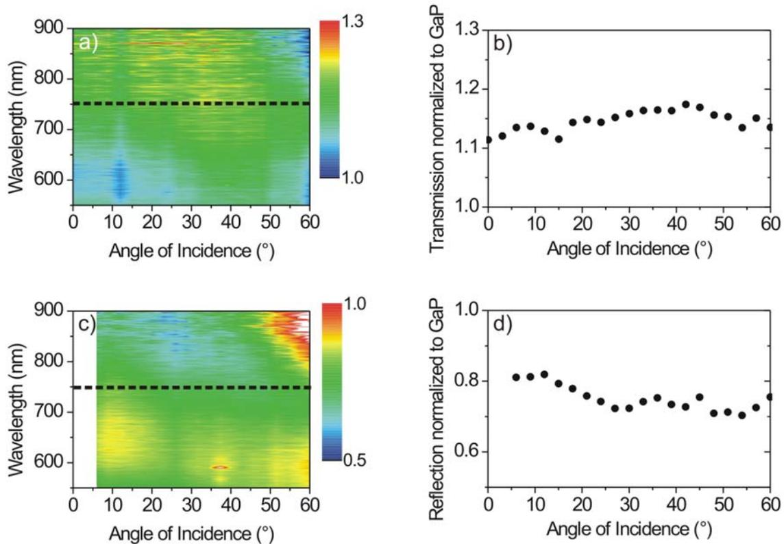
**Figure 5.** a) Angular dependent transmission and c) reflection of a layer of GaP nanorods of sample II normalized to the transmission and reflection of a bare GaP substrate. b) and d) show the transmission and reflection measurements at 750 nm (along the dotted lines of a) and c)).
