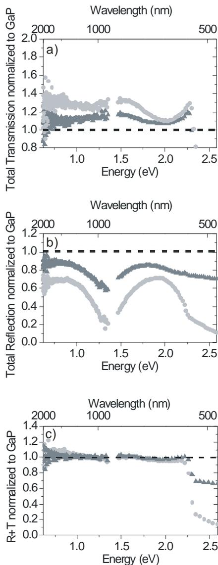
**Figure 4.** Total transmission a) and total reflection b) of sample I (light grey circles) and II (dark grey triangles) normalized to the measurements on a GaP substrate. c) Sums of the total
