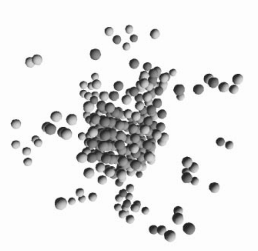
FIGURE 4.2 Snapshot of all solid particles in the r^{-12.5} system at the precritical side of the nucleation barrier, at 25% supercooling ( P = 22.54 , T = 0.75 ). The size of the large solid cluster in the middle is 150 particles.
