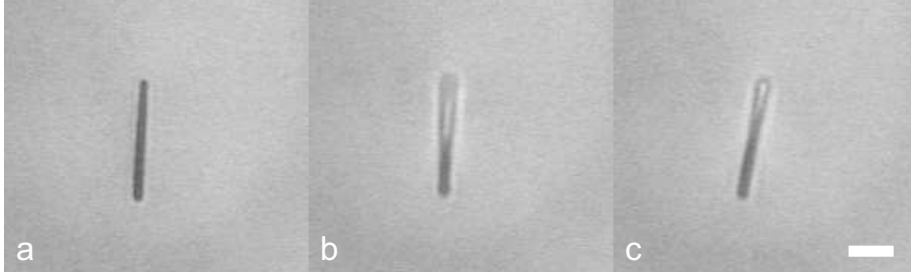
Fig. 6.4: A silica-coated Si rod in water, trapped in counter-propagating line tweezers (a) against the bottom surface, and (b) 8 \mu\text{m} above the bottom surface, where it is (c) rotated over 10^\circ . Scale bar is 2 \mu\text{m} .
