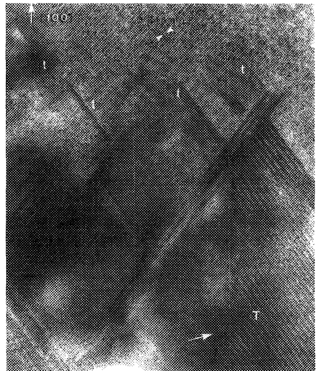
FIG. 9. High-resolution image of solidification structures shown in Fig. 7(a): interface between region I and II. Twins are indicated "t" and "T".
