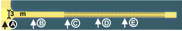
Figure 5.1: Optical microscope image of the structure under investigation. At the bottom, a SPP launch pad is visible. After the tapered entrance a 3 \mu\text{m} wide SPP entrance guide is created. A 55 \mu\text{m} long Bragg grating is fabricated in continuation of the entrance guide. The Bragg grating consists of an arrangement of 1.25 \mu\text{m} indentations with a period of 750 nm, leaving a 500 nm Au strip remaining at the center. Arrows plus letters indicate measurement positions used in figure 5.2 and figure 5.5.
