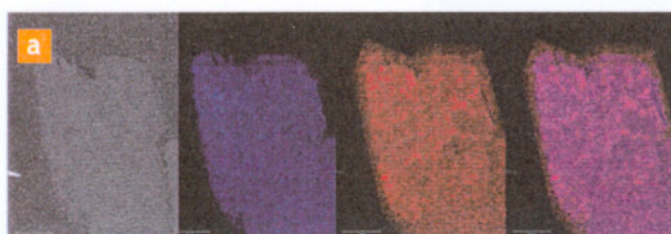
Figure 1 | Sagittal sections of a rat brain (collaboration with Organon, Scotland). Left (fig 1a): from left to right an optical image of a section covered with DHB and coated with 2 nm gold afterwards, followed by MS images of 2,5-dihydroxybenzoic acid (DHB) ( M+H , 155 m/z ), Au^+ (196 m/z ) and their overlay (scale bar 2 mm). The DHB image (in blue) exhibits very sharp contours corresponding exactly to the brain shape, whereas the gold image (in red) seems homogeneous on the whole measured area. The red fringe on the overlay of the two previous images highlights the sole presence of gold
