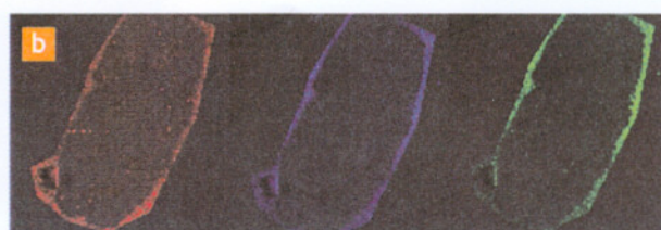
signal at the periphery of the tissue on the glass itself, whereas the matrix peak appears exclusively on the tissue. Right (fig 1b) brain section covered with sinnapinic acid (SA). From left to right, MS images of protonated SA ( M+H , 225 m/z ), sodiated SA ( M+Na , 247 m/z ) and with potassium ( M+K , 263 m/z ). The matrix peaks appear with a highest intensity from the glass, with hardly any signal coming from the tissue.
