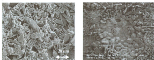
Figure 2 | Electron Microscope images of the matrix crystal layer applied on breast cancer tissue with the ImagePrep apparatus (Bruker Daltonik). Crystal sizes range from 2 to 20 microns. Right panel shows a hole drilled into the same matrix by laser pulses. Laser diameter is much bigger than the crystal size but, in ion-microscope mode imaging, the crystal size limits the spatial resolution.
